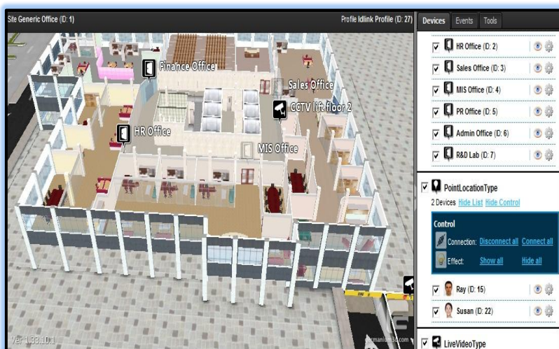
Typical 3D Office Building view with integration to Access control system, GPS locationing and CCTV Camera
